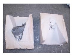
The above photos demonstrate resistance to aluminum metal melted in a test crucible.
